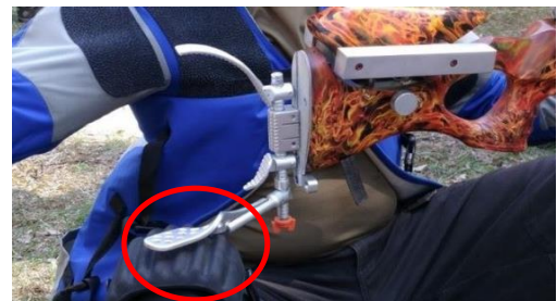
Figure 2 - Rear Stock or/and Butt hook modified to add an additional body support
